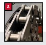
4" double pitch roller chain has 70,000 lbs. pull strength per side for heat and oil resistant belt. a total 140,000 lbs. pull strength.
