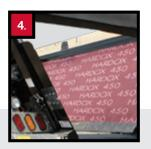
Our hopper bodies inside sheating comes standard with 1/8" 450 Hardox material. Our seal plates are also made of the same material.
