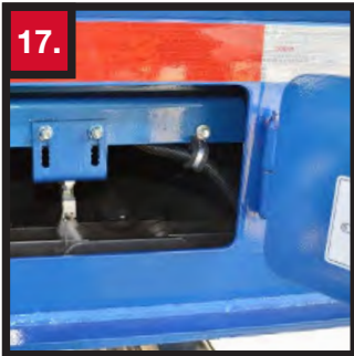
CONVEYOR INSPECTION DOOR Convenient locations to visually inspect and/or access conveyor.
