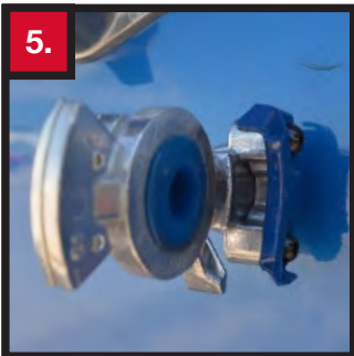
5. SERVICE GLAD HAND Service Glad hand (blue) used to connect air brake service air supply lines between the truck and the trailer.
