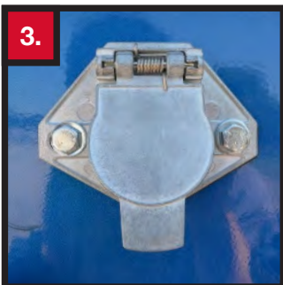
3. AUXILIARY- 7 WIRE PLUG Auxiliary 7 wire electrical connection provides power for components such as Tailgate Lift & Locks, Strobe & Work lights, Strobe Lights, Back Up Alarm, Lift Axle(s), and Air Suspension Dump.
