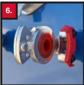
6. EMERGENCY GLAD HAND Emergency Glad hand (red) used to connect emergency air supply lines between the truck and the trailer.
