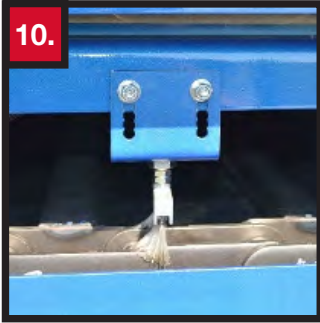
10. OIL BRUSHES Stainless Steel rounded shank brush to apply hydraulic oil to conveyor chain links.
