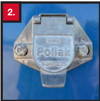
2. STANDARD-7 WIRE PLUG Standard 7 wire electrical connection provides power for trailer lighting functions including clearance/marker lights, stop/turn/tail lighting and ABS power.
