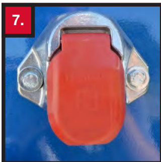
7. ELECTRIC TARP PLUG Electric Tarp plug with 2-pole socket that provides tarp motor ground and power functions.
