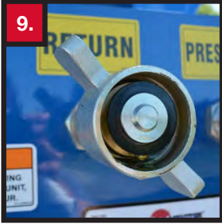
9. HYDRAULIC RETURN LINE Return line should always be connected first to help avoid damage to the hydraulic components. Keep area clean.
