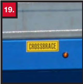
CROSS-BRACE Cross-brace indicators identify the location of the horizontal cross-brace(s) that run across the top of the trailer.
