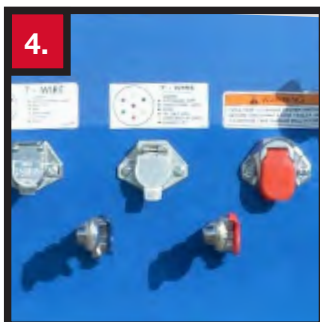
4. CONNECTION PLATE Front plate where all the truck/trailer connections are located: hydraulic pressure & return lines, service and emergency glad hands, main & auxiliary electrical 7-wire connections, electric tarp plug and hydraulic pressure gauge (optional).
