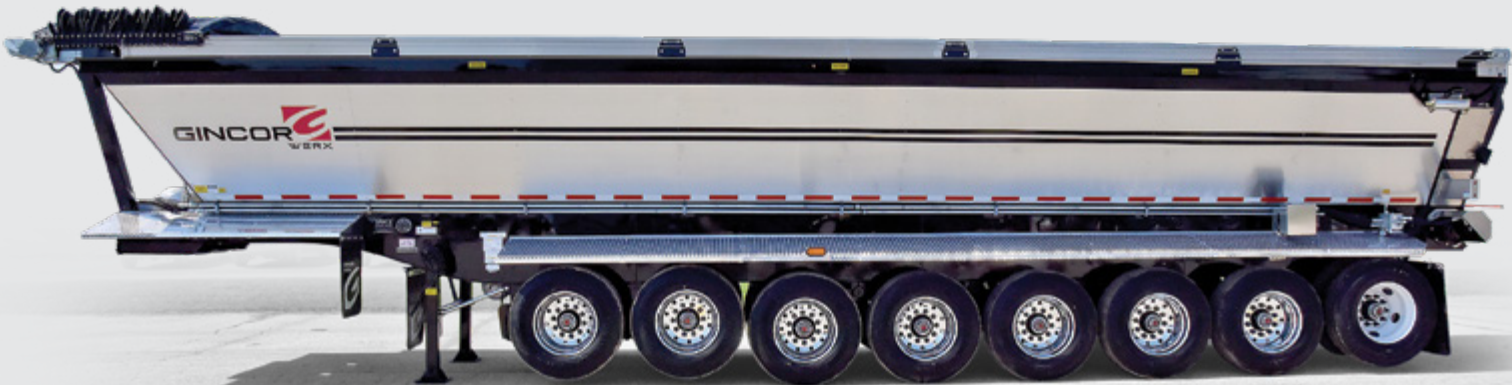
4. Our hopper bodies inside sheathing comes standard with 1/8" 450 Hardox material. Our seal plates are also made of the same material.
