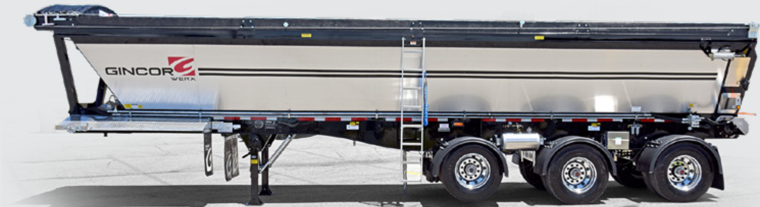
4. Our hopper bodies inside sheathing comes standard with 1/8" 450 Hardox material. Our seal plates are also made of the same material.
