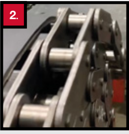
2. 4" double pitch roller chain has 70,000 lbs. pull strength per side for a total 140,000 lbs. pull strength.
