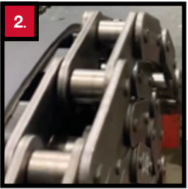
2. 4" double pitch roller chain has 70,000 lbs. pull strength per side for a total 140,000 lbs. pull strength.
