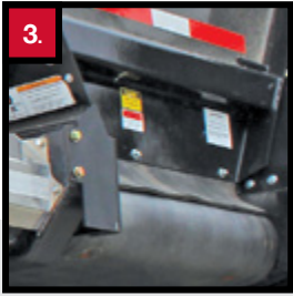
3. Standard 3/8"Goodyear chain has 70,000 lbs. pull strength per side for a total 140,000 lbs. pull strength.
