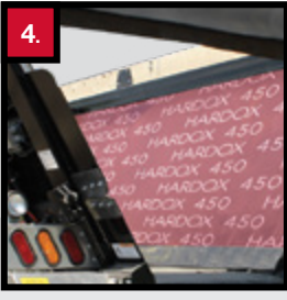
4. Our hopper bodies inside sheathing comes standard with 1/8" 450 Hardox material. Our seal plates are also made of the same material.
