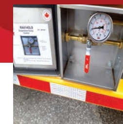
Raise and dump valve with gauge in a stainless steel box.
